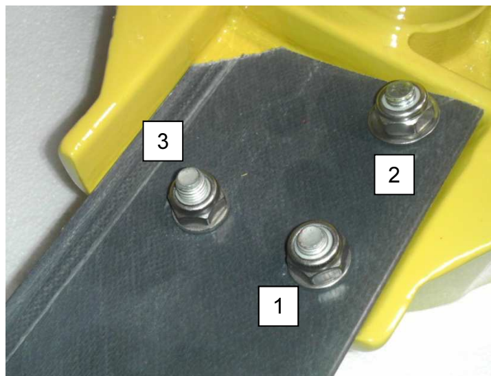
Figure 12: Nut Tightening Order
