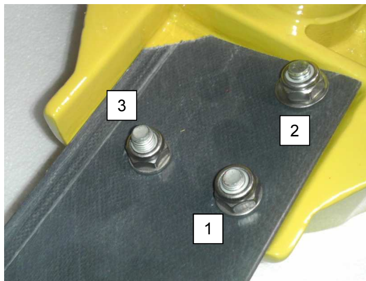
Figure 12: Nut Tightening Order
