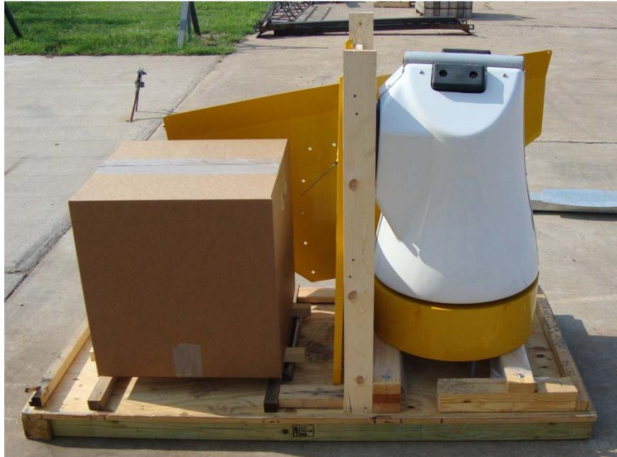
1. Powerhead Skid: 750 lb, 73" x 53" x 35" (HxWxD)
