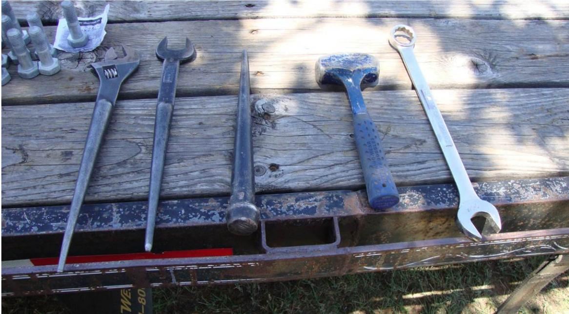
Get the tools ready. To make installation easier, you will want two spud wrenches (one 3/4" and one adjustable, for aligning holes and tightening bolts), a bullpin (to clean out excess zinc), a hammer, and a 3/4" box end wrench.
