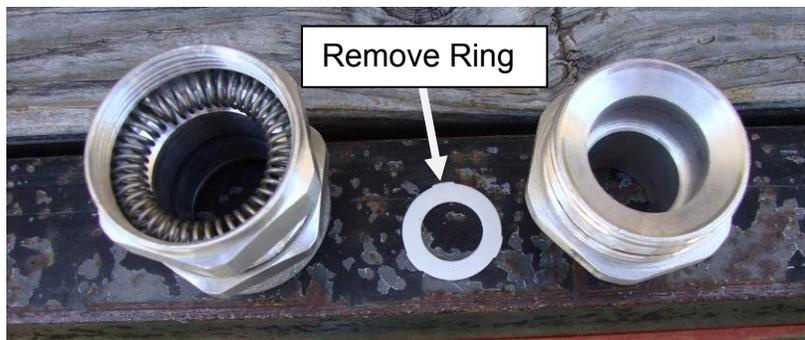
c. It is best to install the connector on the cable before installing the assembly into the junction box. Disassemble the fitting, and remove the plastic ring. Reassemble the fitting.
