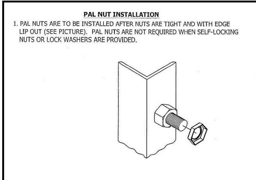
Once the connections have been torqued, apply PAL nuts to the connections that do not have pin-loc nuts.
