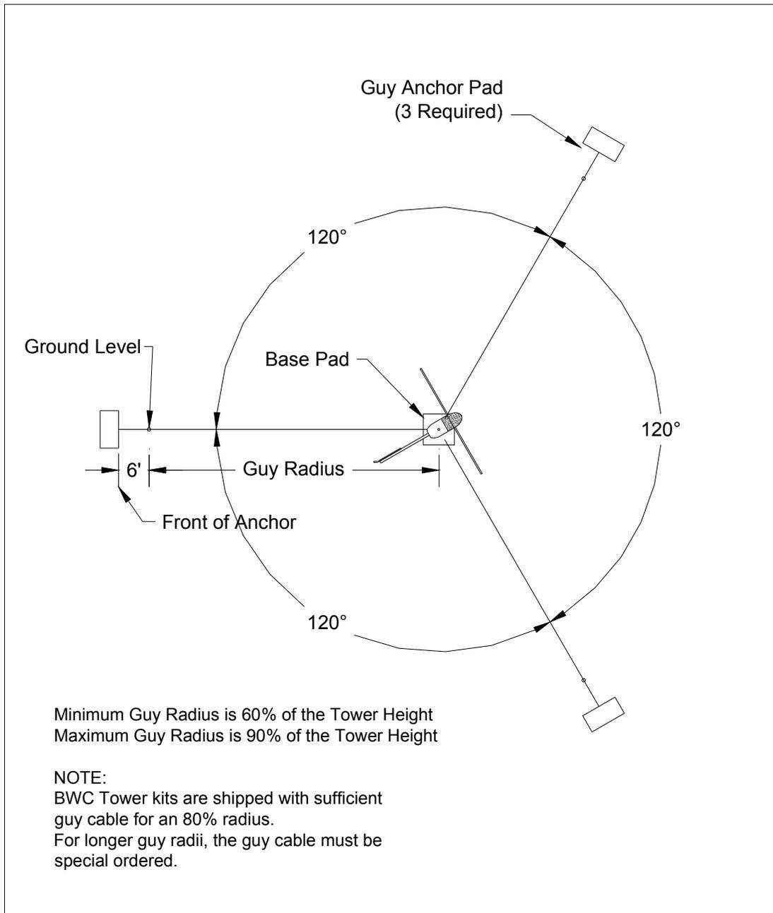
Figure 1: Tower Plan View
